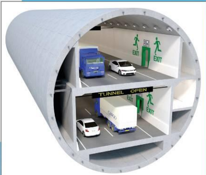
Early Concept Bored Tunnel Cross Section
